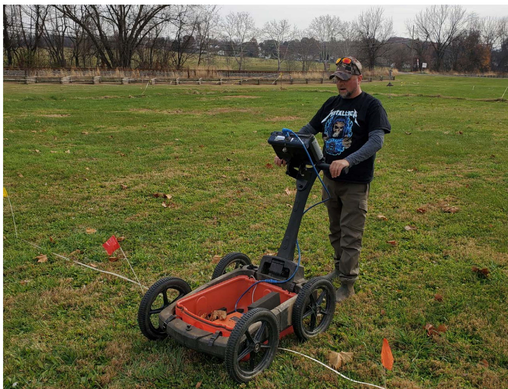
Dr. Burns operating SIR-3000 survey cart with 900 MHz antenna
